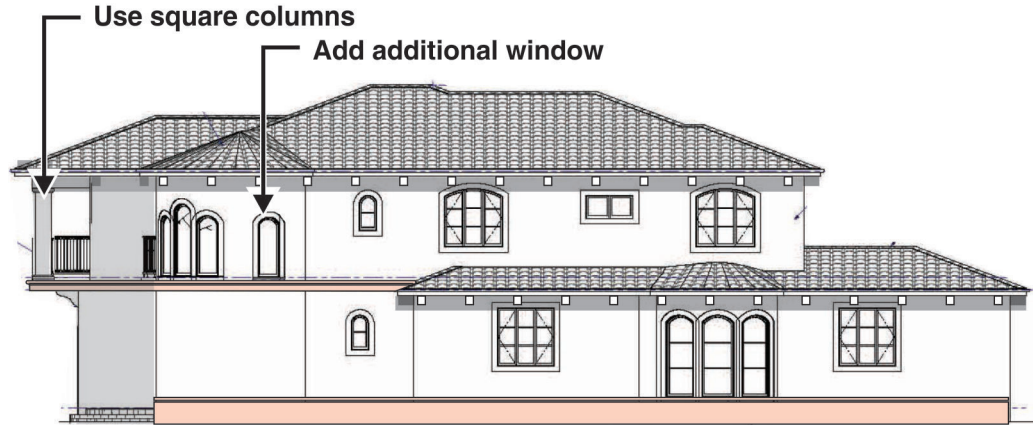
Recommended Shady View Lane Elevation
